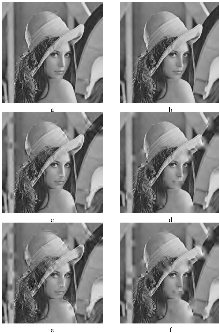
Figure 6.3: Comparison of proposed method (left column) and zerotree style packetization (right column) for the Lena image at 0.208 bpp, (a)-(b) 1% loss, (c)-(d) 10% loss, (e)-(f) 20% loss.
