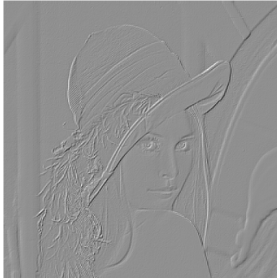
Figure 9.2: The rescaled difference of images Fig. 9.1 (a) and (b). Medium gray levels indicate where the two are identical. The differences are the dark and bright colored areas.
