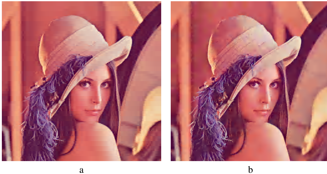
Figure 4.3: Comparison of (a) SPIHT coding using 6 levels of Haar filtering and (b) quadtree-guided encoding. Lena image at 0.24 bpp.
