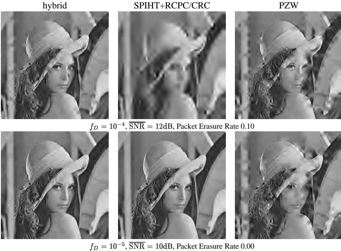
Figure 3. These Images show the median performance of the three algorithms for two channels. Images in the top row were sent across a channel dominated by packet erasures. The channel for the bottom row of images was a slow-fading low-power channel (high probability of bit errors in long bursts) with no packet erasure. Overall transmission rate was 0.25bpp.
