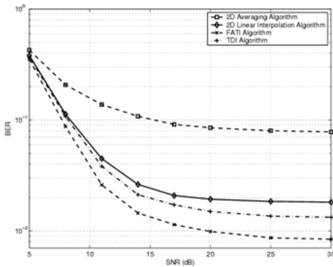
Figure 6. Bit error rate (BER) performance versus SNR, for a WiMAX system operated with the bandwidth  $BW=500\text{MHz}$  and the center frequency  $f_c=60\text{GHz}$ , with a highway speed of the MS  $v=70\text{mph}$
