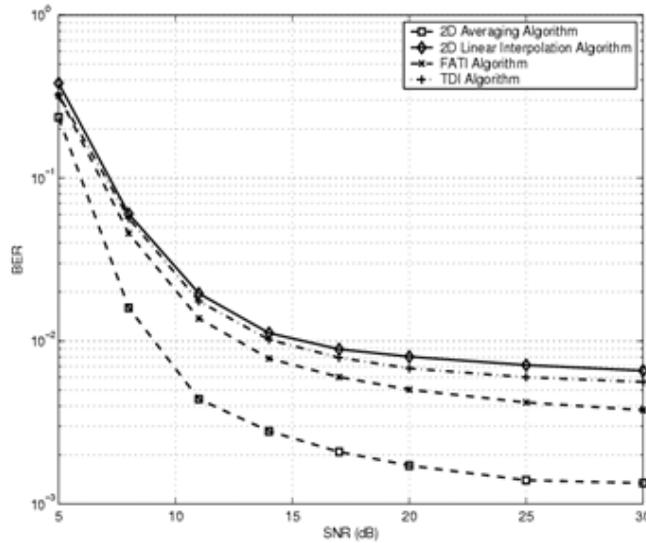
Figure 5. Bit error rate (BER) performance versus SNR, for a WiMAX system operated with the bandwidth  $BW=10\text{MHz}$  and the center frequency  $f_c=60\text{GHz}$ , with a local speed of the MS  $v=35\text{mph}$
