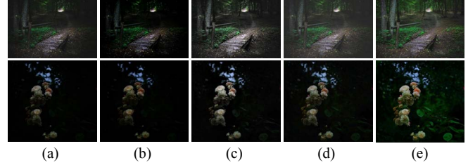
Fig. 3: Restoration of dimly lit images: (a) Original images. The restored images obtained by (b) [2], (c) CLASH [21], (d) gamma correction ( \gamma = 0.75 ), and (e) the proposed method with A^c = 0 . The images are from [27, 28].
