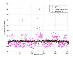
**Fig. 1.** PSNR and three flicker metrics versus frame number for the CZP image encoded with JPEG2000 (EBCOT) at 0.125 bpp.
