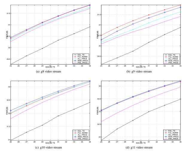
Fig. 2. PSNR variation with bitrate for four multiplexed video streams ( $\alpha_p = 0.1, \bar{p} = 1$ )
