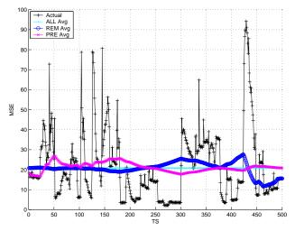
**Fig. 1**. Actual and average MSE variations with TS for g11 video at 50 kbits per TS
