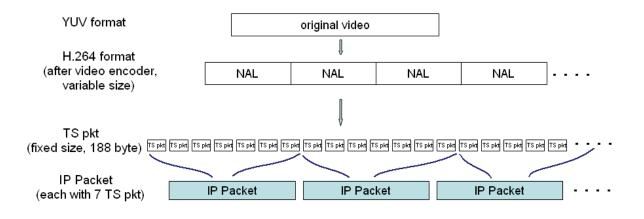
Fig. 1. The encoding and packetization procedure from original video to IP packets.
