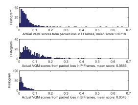
Fig. 5. Histogram of VQM scores from different frame types.
